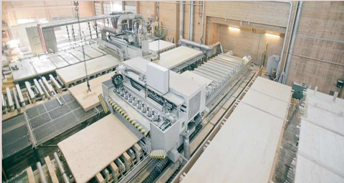
image: 5 axis CNC panel machining center of KLH Massivholz GmbH, Katsch an der Mur
